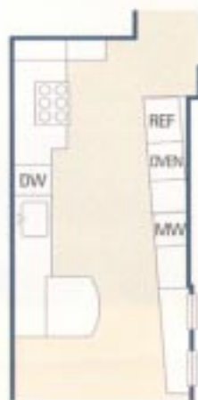
BELOW: The angled wall of appliances and cabinets relieves any 90-degree boredom. The taper also allows a healthy distance between peninsula and seating area.
